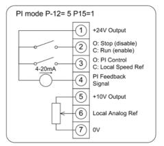
Control set by pressure level Speed set by potentiometer
